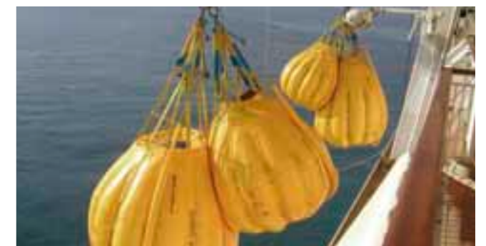
Waterbags for overload test of davits
