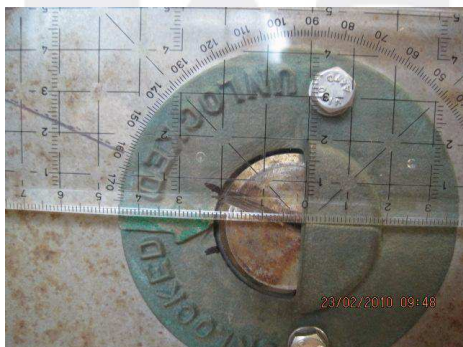
Current Version with open bowden wire and bowden wire lever plates connect with screws; release bolt angle about 30 – 35°
